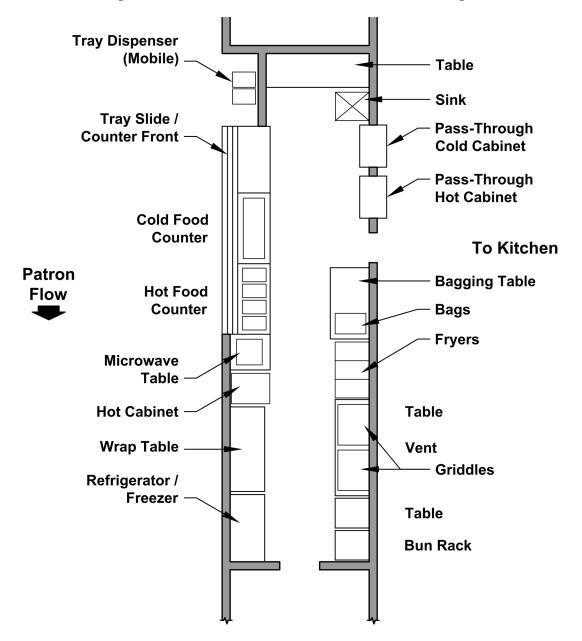
Figure A-6 Schematic Plan of Fast Food Serving Line
