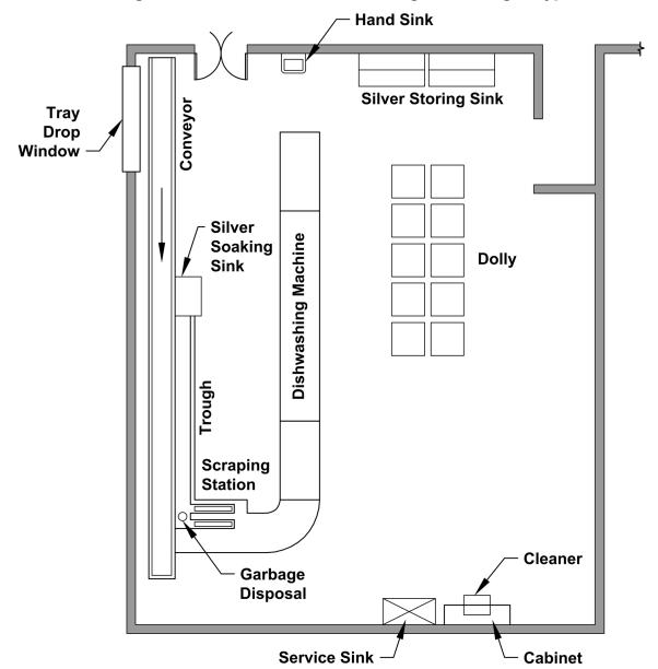
Figure A-13 Schematic Dishwashing Plan – Flight Type
