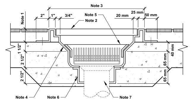
Figure A-28 Sump Drain - Pan Type
