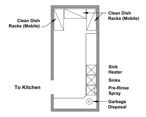
Figure A-15 Schematic Plan of Mechanical Utensil Washing
