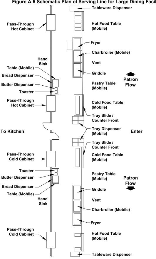
Figure A-5 Schematic Plan of Serving Line for Large Dining Facility
