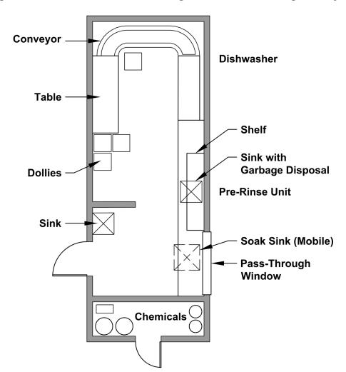
Figure A-11 Schematic Dishwashing Plan Medium Dining Facility
