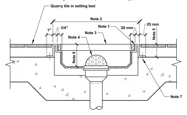
Figure A-29 Sump Drain - Tile Type
