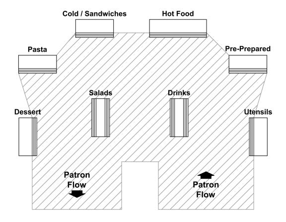
Figure A-32 Schematic Plan of Horseshoe-Shaped Serving Line
