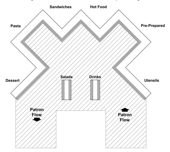
Figure A-34 Schematic Plan of Sawtooth-Shaped Serving Line
