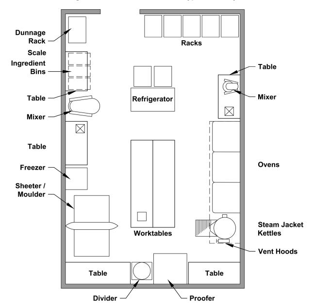
Figure A-20 Schematic Plan of Typical Bakery
