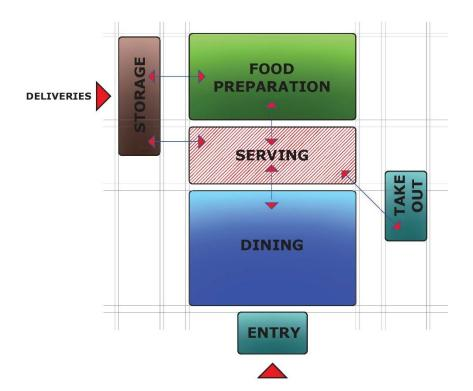
Figure 2-1 Dining Facility Flow Schematic
