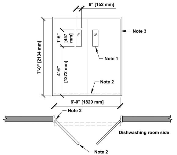
Figure A-24 Double Doors at Dishwashing Station
