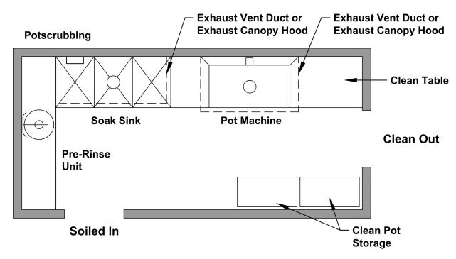
Figure A-16 Schematic Plan of Kitchen – Small Dining Facility (Pot Cookery)
