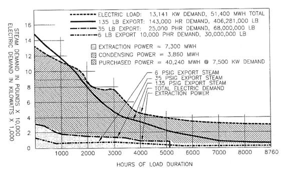
Figure H-4 Typical Load Duration Curves
