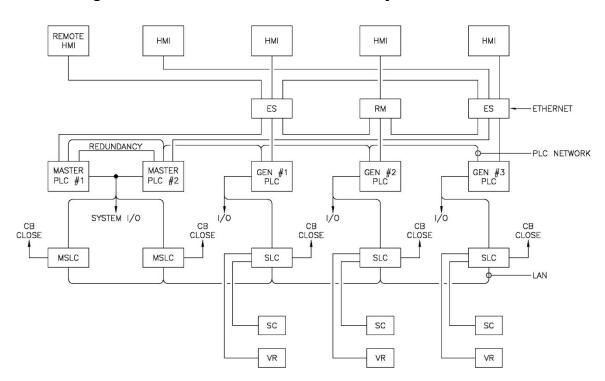
Figure B-10 Parallel Generator Control System Architecture
