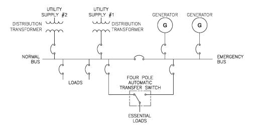
Figure B-9 Parallel Generators with Alternate Utility Supply for UPS Systems
