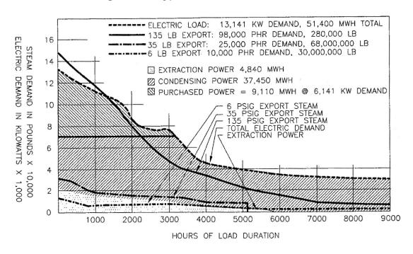
Figure H-3: Typical load duration curve - base load on power plant, load swings on purchased power, portion of export steam on central heating plant.
