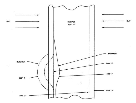
Figure 4-7 Effect of Boiler Deposits on Boiler Tube
