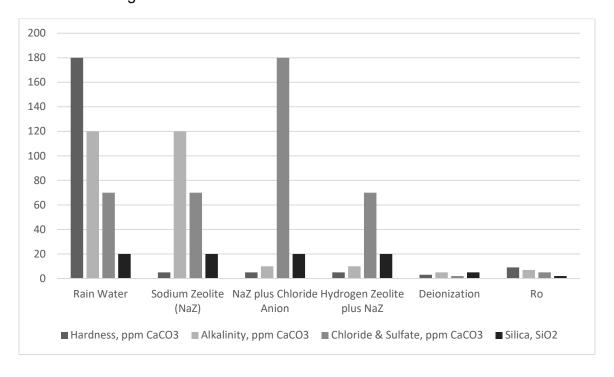
Figure 3-1 Effects of Treatment on Raw Water
