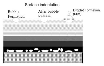
Figure 4-15 Water Boiler Mist Formation
