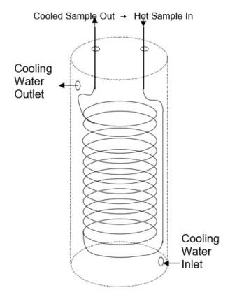
Figure 7-2 Boiler or Condensate Water Sample Cooling Coil.
