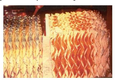
Figure 5-14 Heavily Fouled Cooling Tower Film Fill
