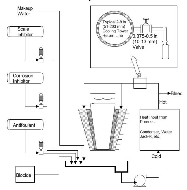
Figure 7-1 Typical Water Sampling Points for an Open Recirculating Cooling Water System
