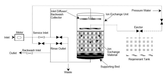
Figure 3-2 Typical Ion Exchange Unit
