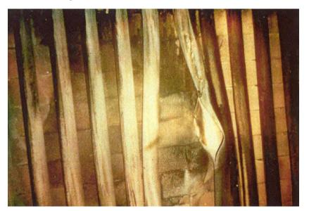
Figure 4-9 Failed Boiler Tube
