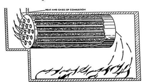
Figure 4-1 Fire Tube Boiler
