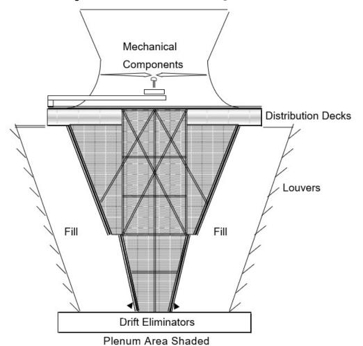
Figure 5-6 Cross-Flow Cooling Tower
