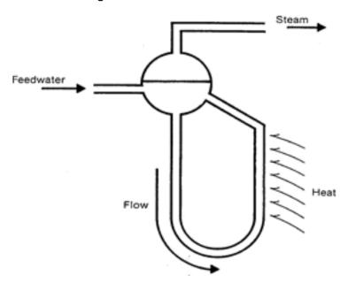
Figure 4-2 Water Tube Boiler
