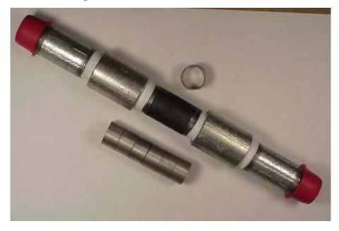
Figure C-1 Condensate Corrosion Tester
