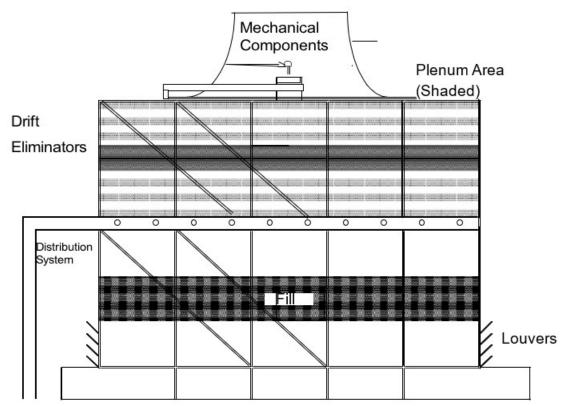
Figure 5-8 Counter-Flow Cooling Tower Diagram
