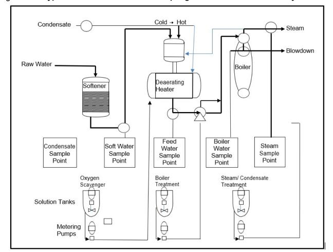
Figure 7-3 Typical Locations for Water Sampling in a Steam Boiler Water System
