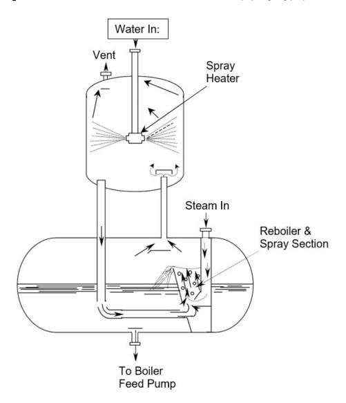
Figure 4-12 Mechanical Deaerator Schematic (Spray Type)
