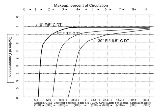
Figure 5-15 Effect of COC on Makeup Requirement
