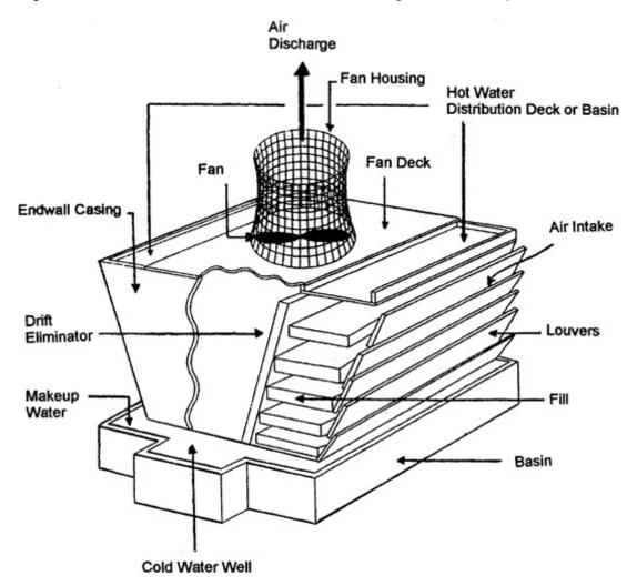
Figure 5-10 Induced-Draft Cross-Flow Cooling Tower Components
