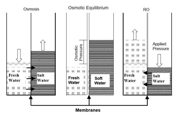
Figure 3-7 RO Schematic
