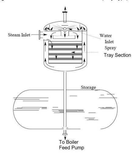
Figure 4-13 Mechanical Deaerator Schematic (Tray Type)
