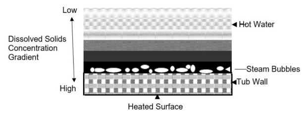
Figure 4-11 Localized Scale Formation Process
