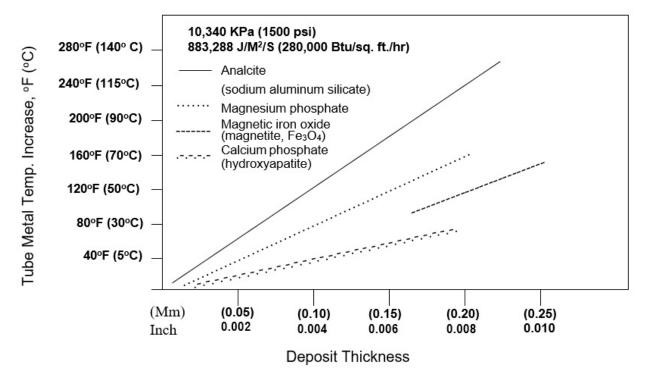
Figure 4-6 Impact of Scale on Heat Transfer
