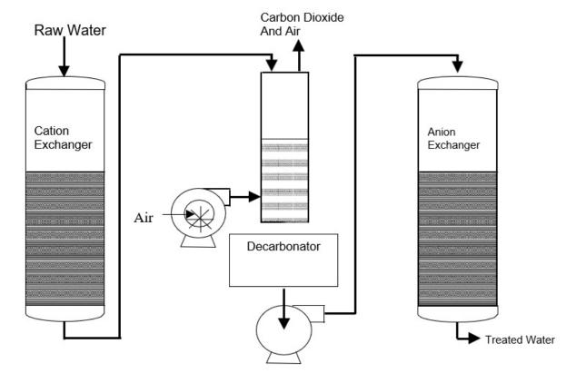
Figure 3-4 **Demineralization Process**
