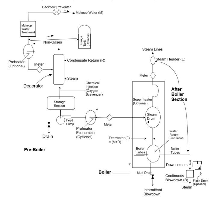
Figure 4-3 Components of a Simple Steam Boiler System
