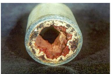
Figure 4-5 **Scaled Boiler Tube**
