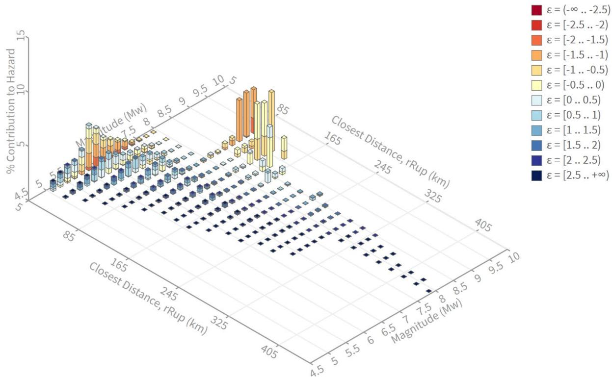
**Figure 4-2.** Hazard deaggregation for 5%-damped, 1-second elastic spectral acceleration response with 20% exceedance probability in 50 years
