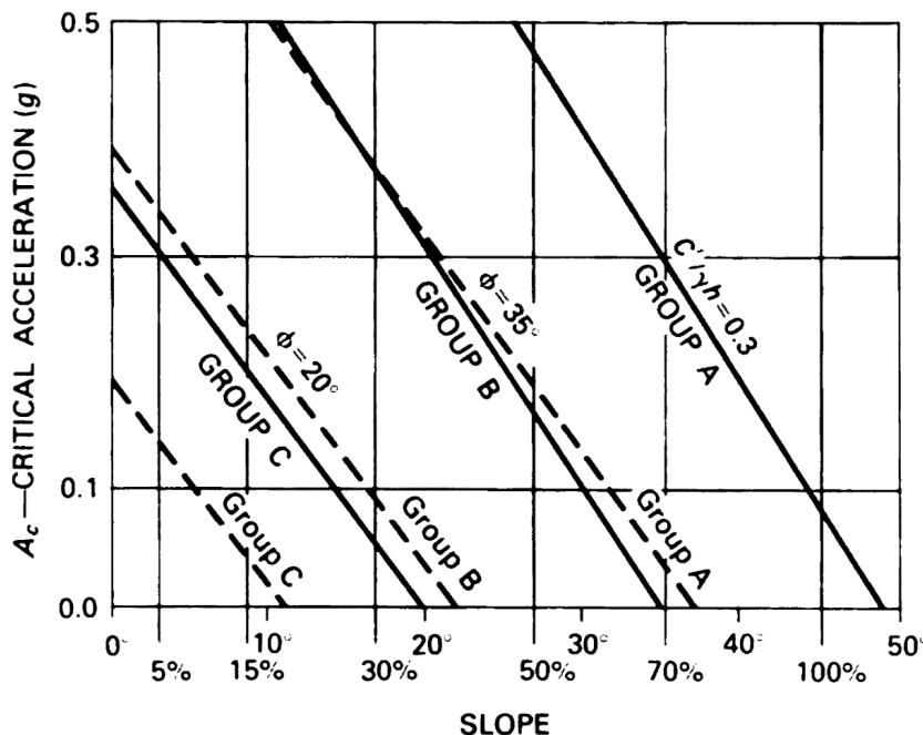
Figure 3-2. Wilson and Keefer (1985) plot of critical acceleration versus slope for three geologic groups
