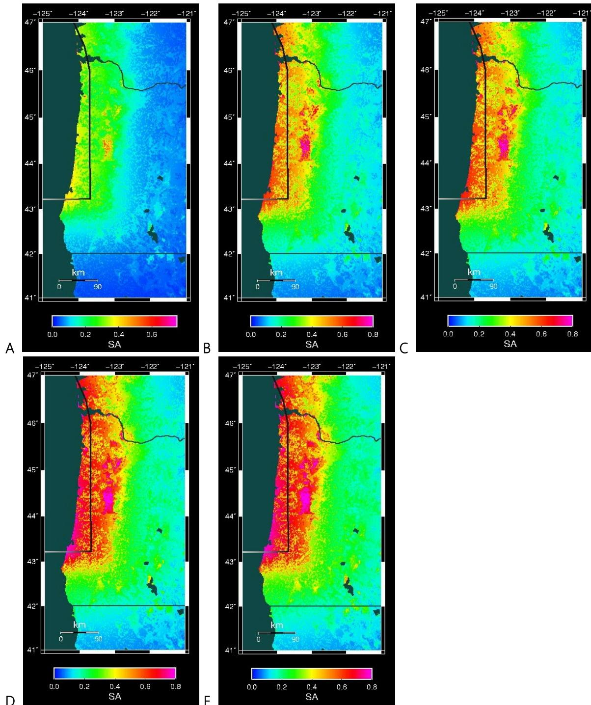
**Figure 5-4.** Damped elastic spectral acceleration response at 1.0-second period in Cascadia megathrust scenarios with 50-year exceedance probabilities of (A) 50%, (B) 20%, (C) 10%, (D) 5%, and (E) 2%
