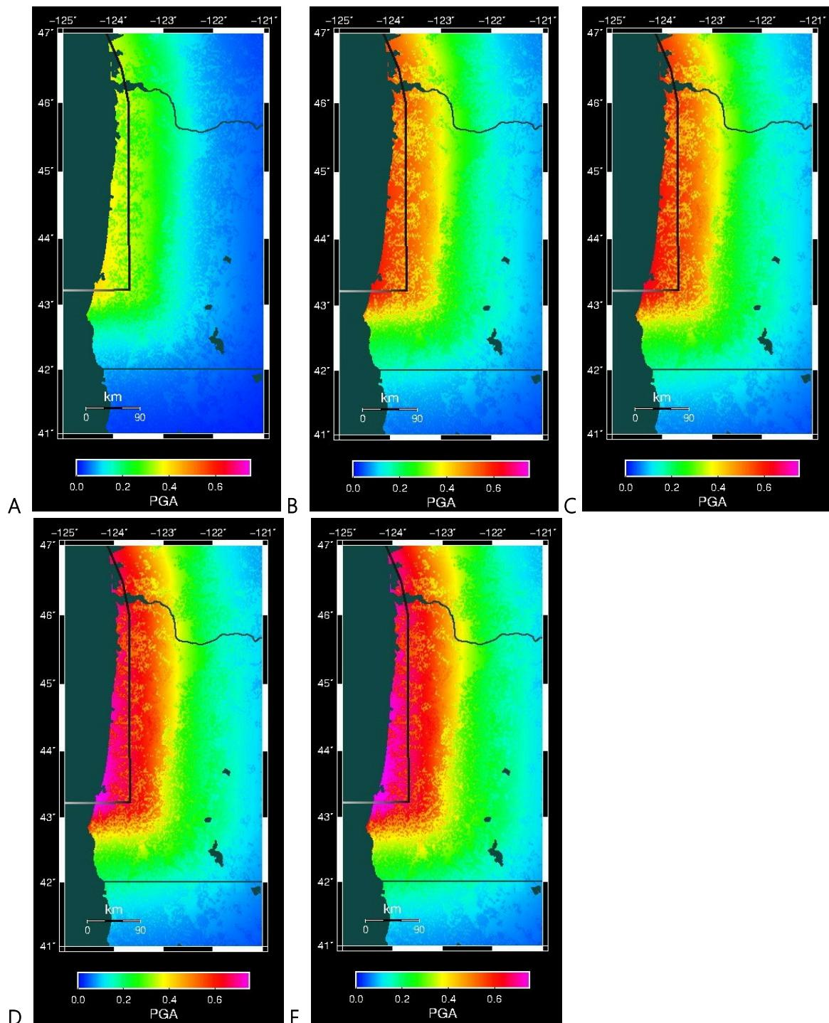
Figure 5-3. Peak ground acceleration (PGA) in Cascadia megathrust scenarios with 50-year exceedance probabilities of (A) 50%, (B) 20%, (C) 10%, (D) 5%, and (E) 2%
