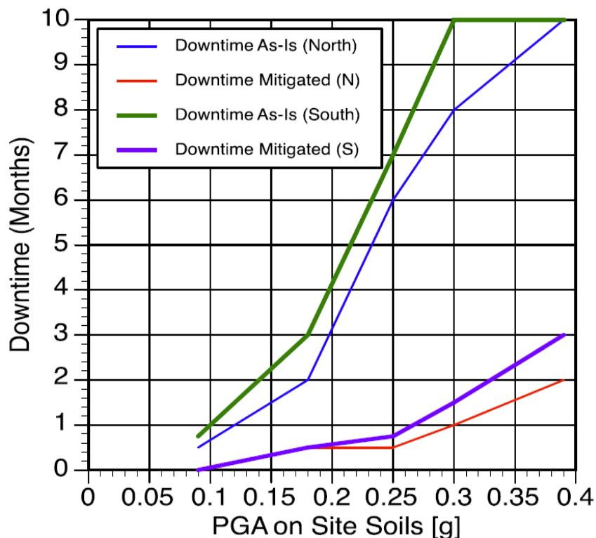
**Figure 5-2.** Estimated runway repair duration as a function of ground motion, as-is and mitigated (HNTB Corporation 2015, p. 49). Only the as-is curves are used.
