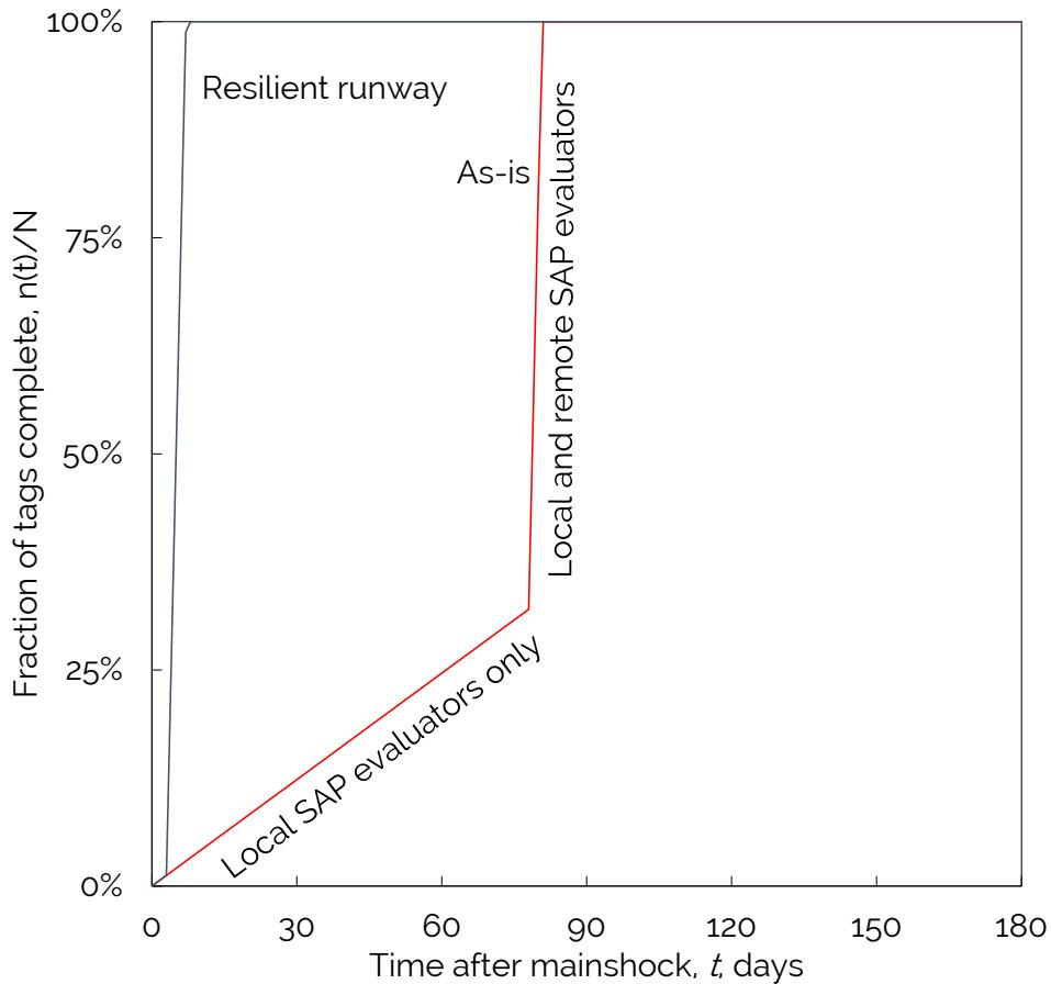
Figure 4-8. Illustration of the effect of a resilient runway on delays in building safety evaluation
