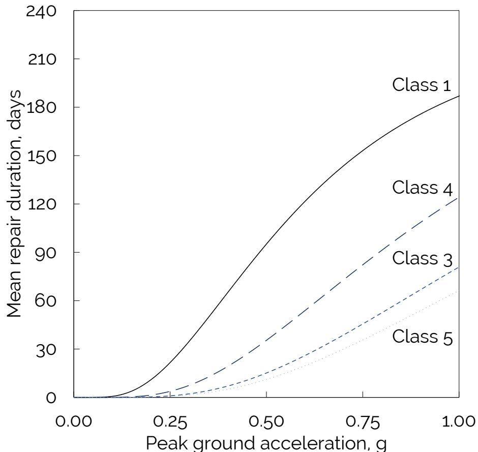
Figure 4-7. Mean bridge repair duration as a function of peak ground acceleration
