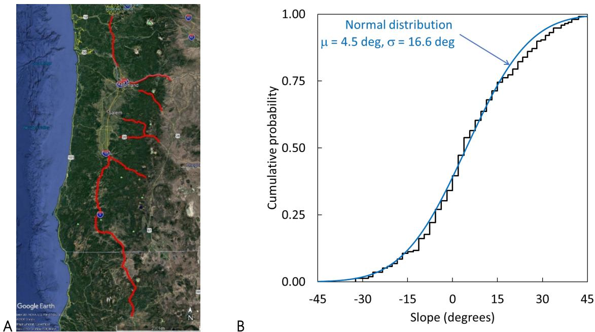
**Figure 5-7.** (A) Seven highway routes through the Cascades to the Willamette Valley; (B) Slope distribution along the route
