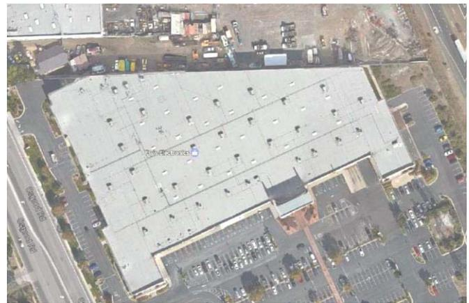
**Figure 2. Structure with non-rectangular diaphragm is beyond the scope of these provisions.**
