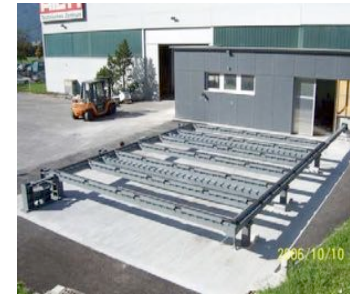
Diaphragm Tests by Industry (e.g. Hilti)
