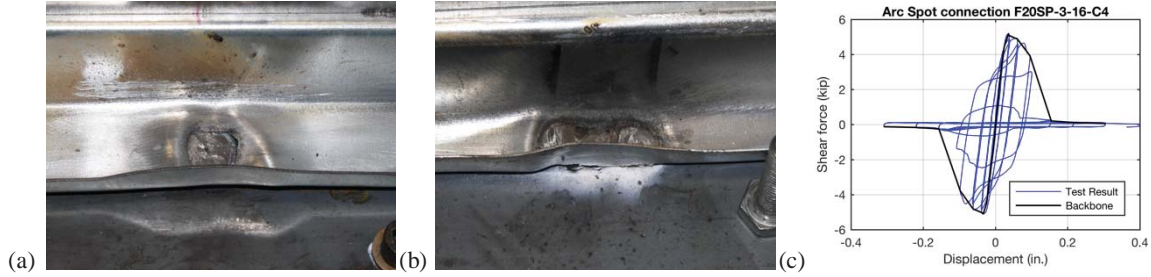
Figure 7: Cyclic shear performance of welds (a) arc spot in 20 gauge deck at failure, (b) arc seam in 22 gauge deck at failure, (c) typical cyclic response of single arc spot weld in 20 gauge deck
