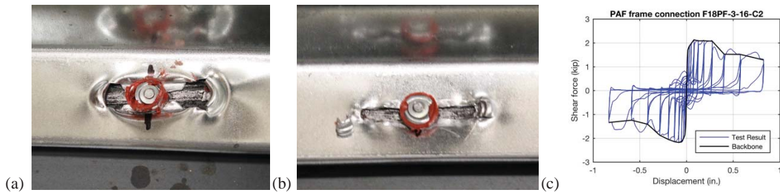
Figure 6: Cyclic shear performance of PAF (a) bunching and damage in 22 gauge deck, (b) slotting and tearing in 20 and 18 gauge deck, (c) typical cyclic response of single PAF in 18 gauge deck
