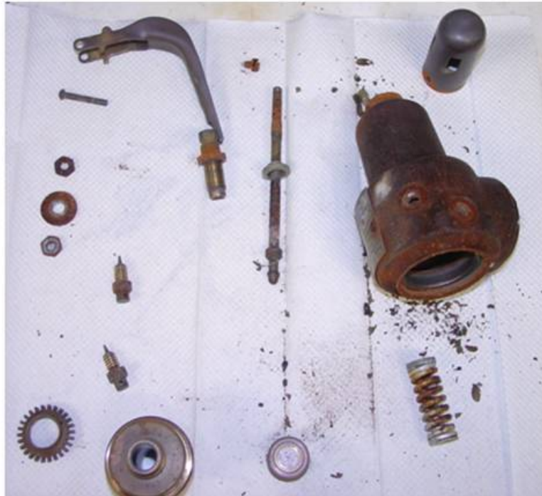
Figure 3.5-1 Corroded Valve Internal
