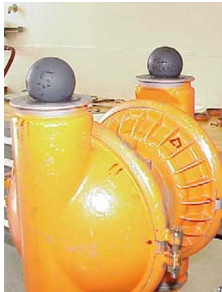
Figure 4.1-2 Removed Discharge Manifold Pipe, Two Check Valves
