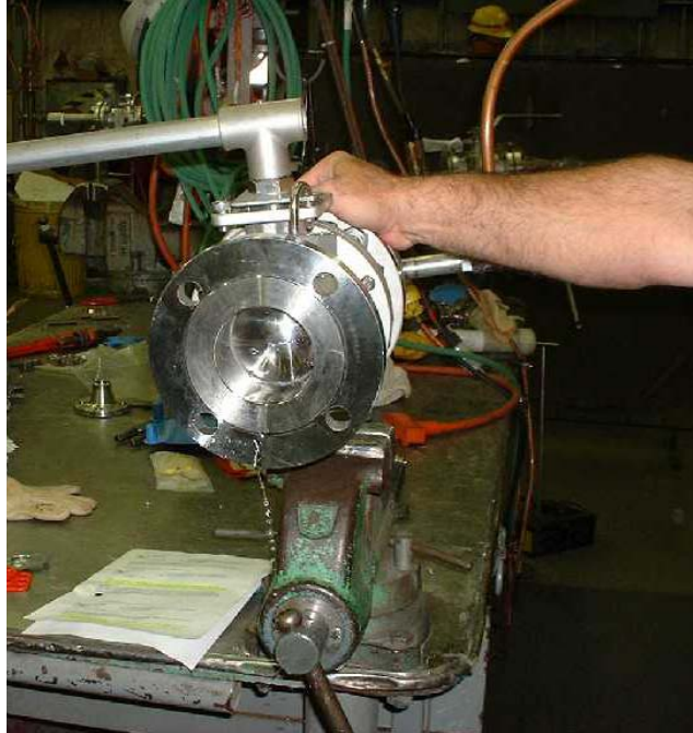
Figure 3.1-1 Through-Seat Leak Test
