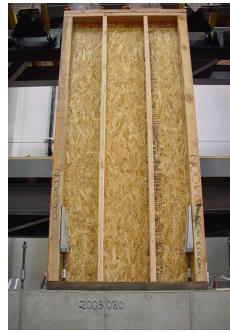
Figure 6.2-1 Engineered shear wall with studs, sheathing, and posts and tie-down connectors at each end.
