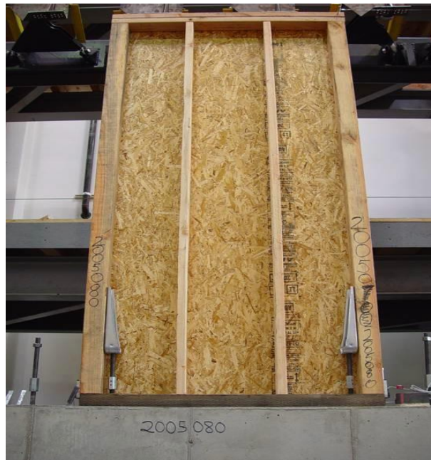
Figure 1.8-1 Segmented shear wall with studs, sheathing, and posts and tie-down connectors at each end (Figure credit: FEMA P-1052)
